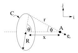
The gravitational field at A is parallel to the axis (by symmetry). Therefore the only component we have to consider is the **i** component.
