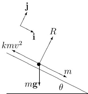
Use the  $\mathbf{i}$  and  $\mathbf{j}$  aligned with the slope and the reaction.
