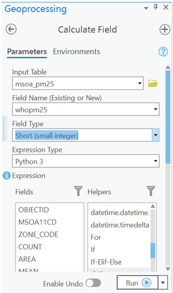
You can then use an ArcPy (Python) function to find those records above 13 micrograms/m<sup>3</sup>. The top box in the screen shot below contains the function, which takes the value of the MEAN field created by zonal statistics as an input (the !MEAN! signifies a field).
