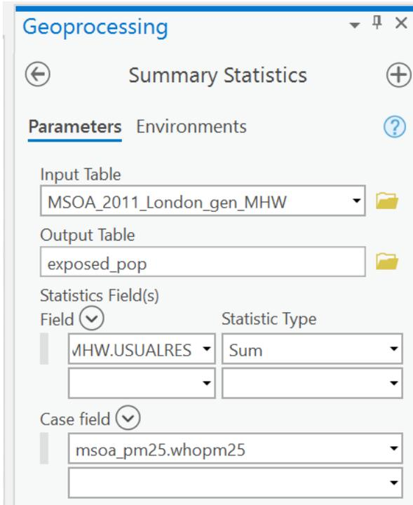
The results are stored in a new table called **exposed\_pop**. Notice the syntax for identifying fields in the joined table: the table name appears first, then the field name, separated by ‘.’.
